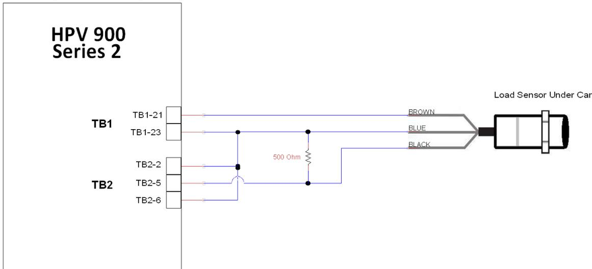
The 900S2 drive uses a -10 to +10VDC voltage analogue input. The resistor is simply to convert a 4-20mA signal to a 3-10V signal which the drive can use.
