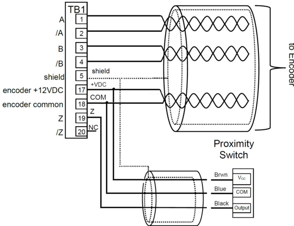
Each of the wires are labelled and should be connected into the TB1 terminals (long connectors). Under no circumstance should any wires be 'switched' away from the labelled order.
