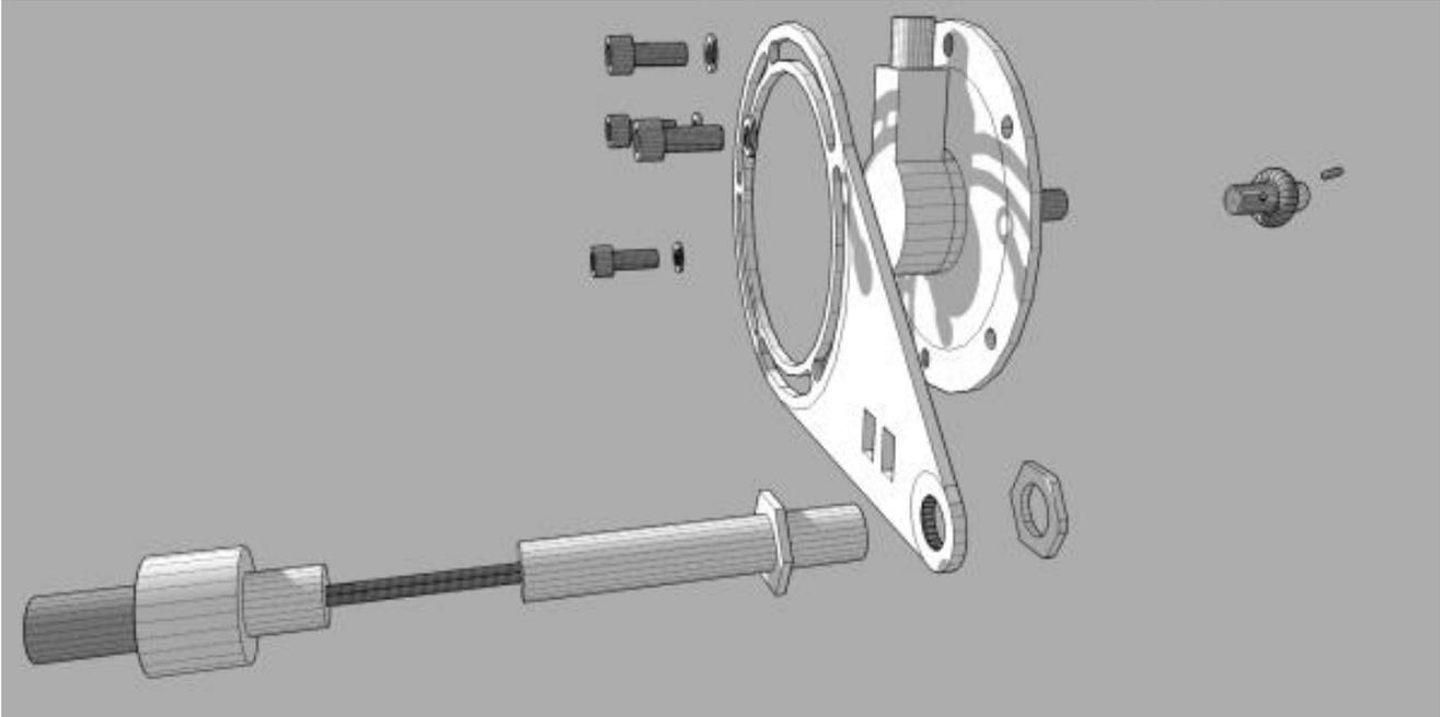
2. The Rider Wheel (supplied as part of the kit) should be attached to the encoder shaft using the grub screws provided. the proximity switch should be fitted to the proximity bracket as pictured below using the supplied nuts.
