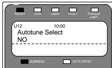
3. Press Enter, and change Autotune select to **ON RUN**. (“Yes” would begin the alignment immediately which would require motor contactors to be bypassed)
