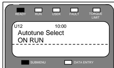
4. Attempt to run the lift on test by pressing the inspection run/direction buttons and keep them depressed whilst the autotune is carried out. During Autotune, a slight buzzing noise should come from the motor for approximately half a second and the RUN light will be lit for the duration of the procedure.
